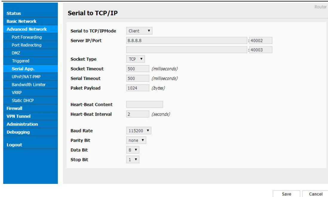
Figure 3-10 Serial App Setting GUI
