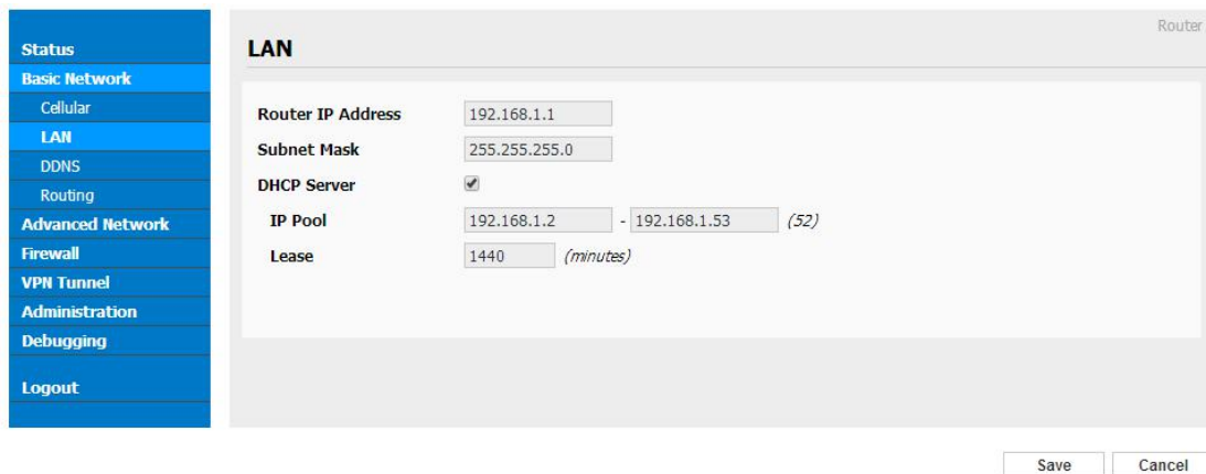
Figure 3-2 LAN Setting GUI
