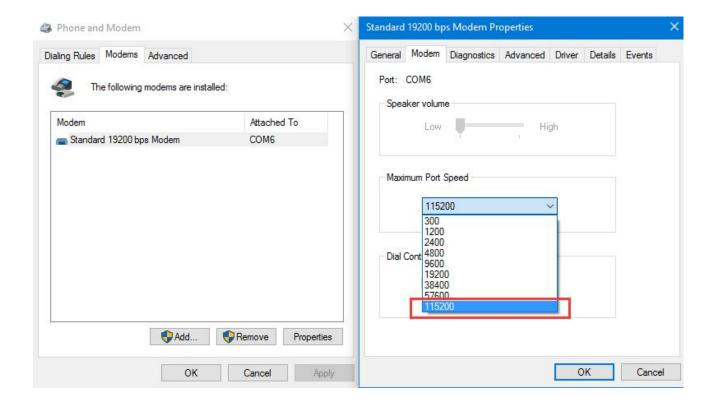
3.3 Click Advanced Button to add Modem dialup command such as at+cgdcont=1,"ip",3GNET". The APN 3GNET should be as the same as SIM card APN in Properties.
