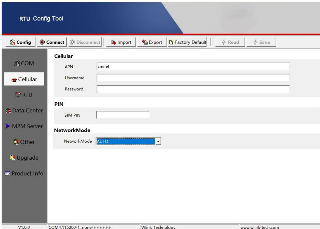
RTU Network settings instruction (In most cases, SIM card will obtain it automatically, no need to setup up)
